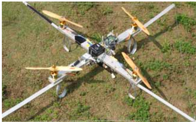
Figure 1: Prototype quad rotor aerial robot with protection jacket.
